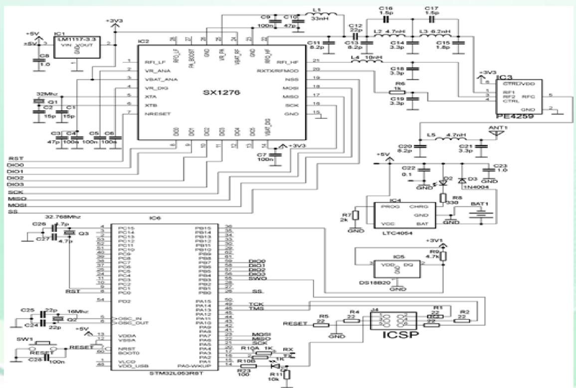
Figure 3. Schematic diagram of the end node
